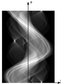
Figure 5.6: A sinogram is a 2D dataset p(r, \theta) obtained by stacking the 1D projections p_\alpha(r) .
