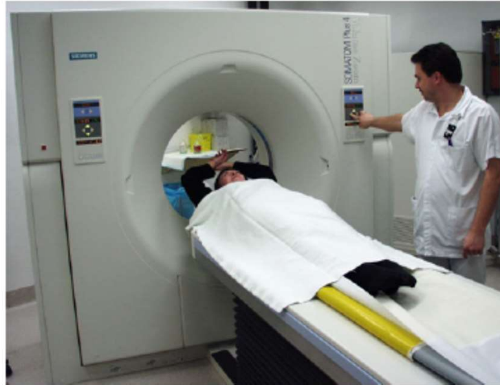
Figure 5.24: Multi-slice CT scanner with four detector arrays (not visible). The external design of a multi-slice scanner is apparently not different from that of a conventional single slice scanner (see figure 5.1).
