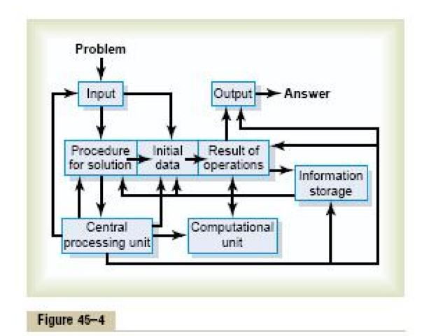
Block diagram of a general-purpose computer, showing the basic components and their interrelations.
